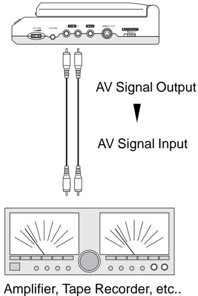
Using only the red and white AV signal cables, the DVD player can provide output signals, for recording or through play. These dual track high-quality audio signals can interface to the following peripherals:
